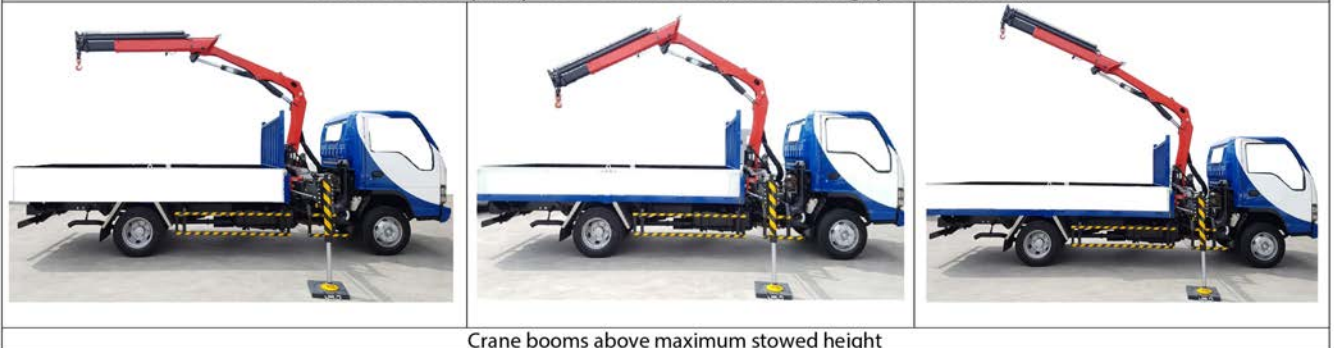
Positions of Inadequately Stowed Crane Boom (Audio Warning System Activated)
