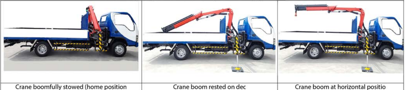
Positions of Inadequately Stowed Crane Boom (Audio Warning System Activated)
